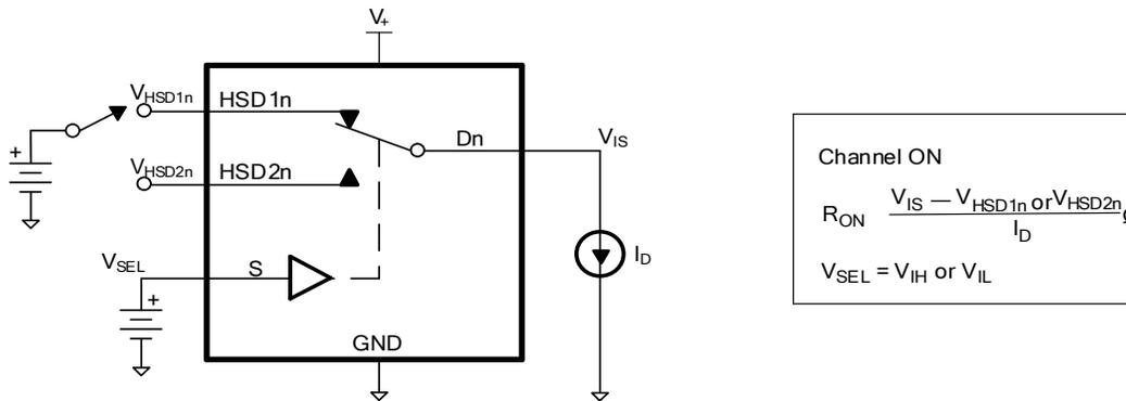
**Test Circuit 1. ON-State Resistance ( $R_{ON}$ )**
