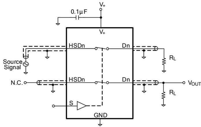
$$\text{Channel To Channel Crosstalk} = -20 \times \log \frac{V_{HSDn}}{V_{OUT}}$$
