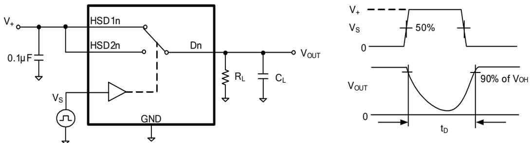
**Test Circuit 3. Break-Before-Make Time ( $t_D$ )**
