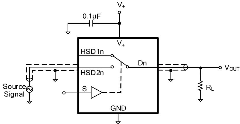
**Test Circuit 4.OFF Isolation (O<sub>Iso</sub>)**
